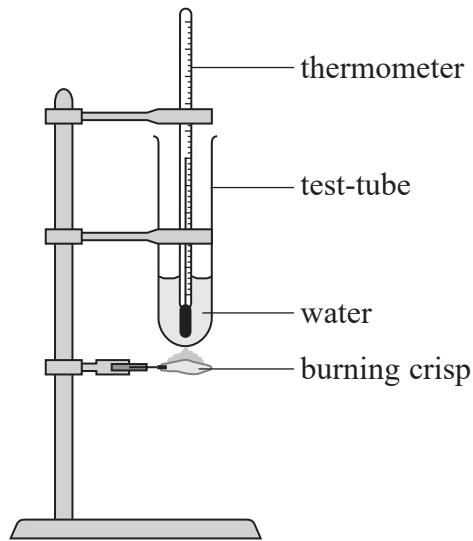
Once the crisp had finished burning, the student recorded the final temperature of the water. The experiment was carried out three times using a crisp of the same mass.
